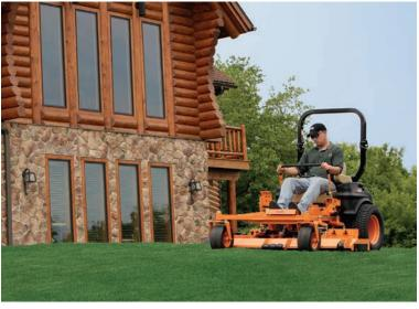
Stay off slopes too steep for safe operation. To check a slope, attempt to back up the slope (with the cutter deck down). If the machine can not back up the slope without the wheels slipping, do not operate the machine on this slope. Under no circumstances should the machine be operated on slopes greater than 15 degrees.
