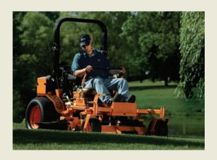
Proper use of a Rollover Protection System (ROPS) with seat belt, along with safe operating practices, has shown to be effective in preventing serious injury or death in the event of an overturn. Be alert, know your surroundings, and watch for hidden obstacles in the work area.
