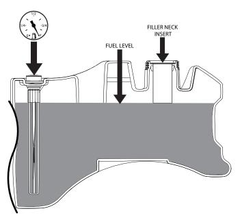
Figure 7-6. C.A.R.B. / EPA Phase 3 Fuel Level
