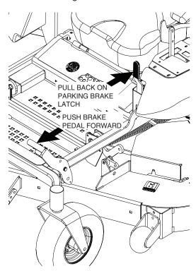
Figure 4-2. Engaging the Parking Brake
