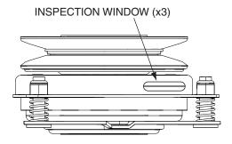
Figure 6-8. Clutch Air Gap Adjustment
