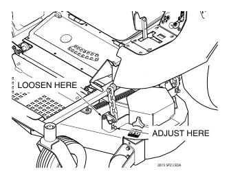
Figure 6-5. Cutter Deck Pitch Adjustment
