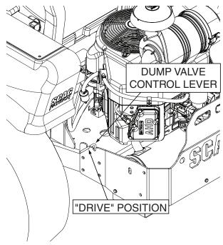
Figure 7-4. Dump Valve Control Lever
