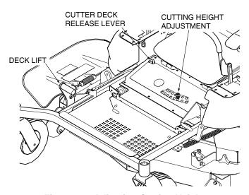
Figure 4-6. Adjusting Cutting Height
