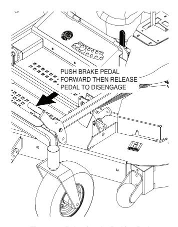
Figure 4-3. Releasing the Parking Brake
