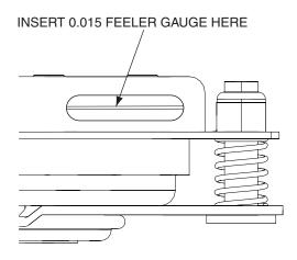
Figure 6-9. Clutch Air Gap Adjustment
