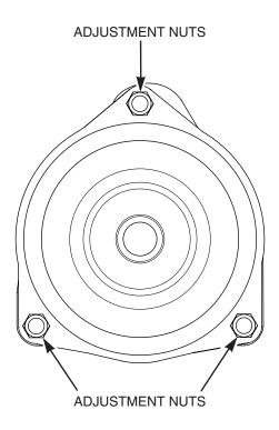
Figure 6-10. Clutch Air Gap Adjustment
