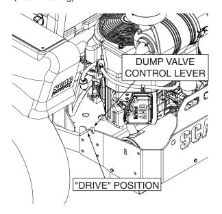
Figure 4-4. Dump Valve Control
