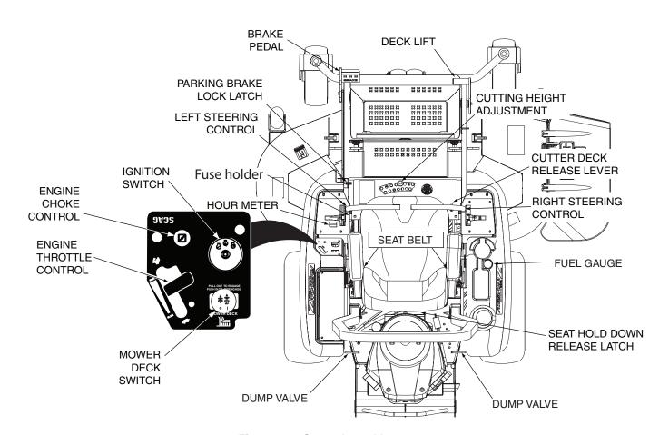
Figure 4-1. Controls and Instruments
