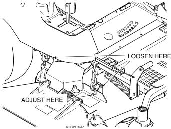
Figure 6-7. Cutter Deck Height Adjustment
