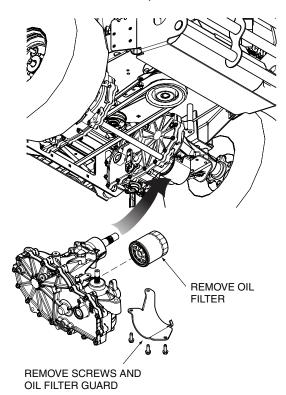
Figure 7-1. Hydraulic Oil Filter and Drain Plug
