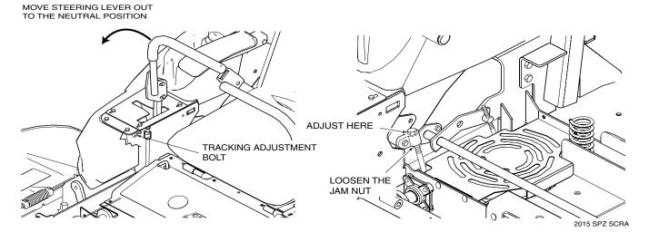
Figure 6-3. Steering Control Rod Adjustment
