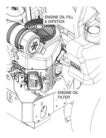
Figure 7-5. Oil Fill / Dipstick, Oil Filter
