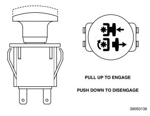
Figure 4-5. Cutter Engage Switch
