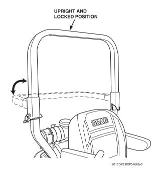
Figure 2-1. Foldable Roll-Over Protection System
