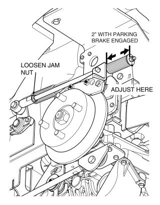
Figure 6-2. Brake Rod Adjustment
