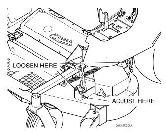
Figure 6-4. Cutter Deck Level Adjustment
