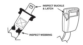
Figure 2-3. Seat Belt Inspection
