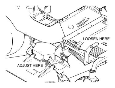
Figure 6-6. Cutter Deck Pitch Adjustment
