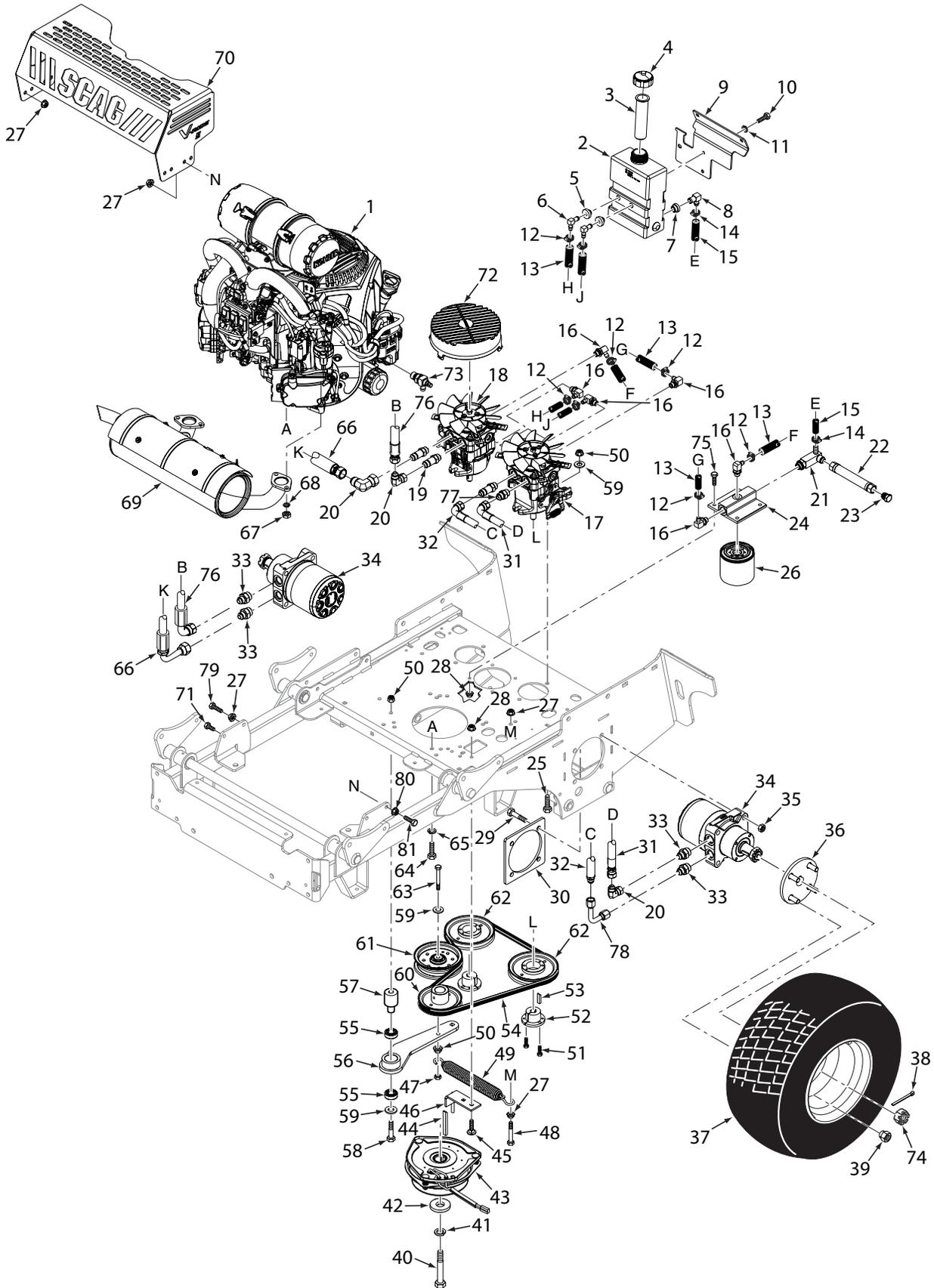
SVRII-48V / 52V / 61V HYDRAULICS AND ENGINE COMPONENTS
