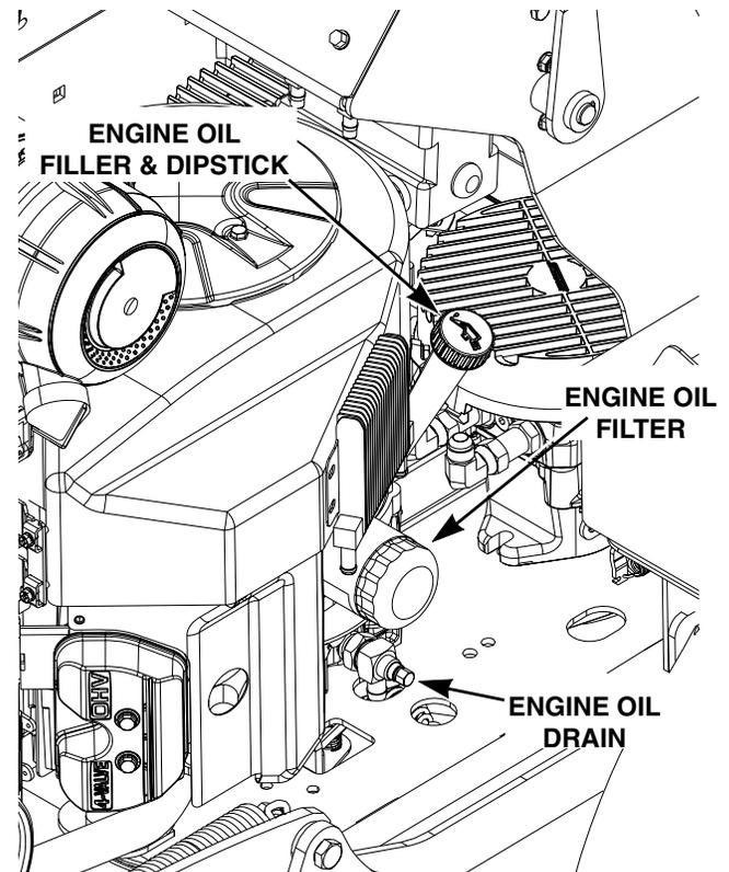
Figure 7-4. Drain Plug, Dipstick and Oil Filter Location
