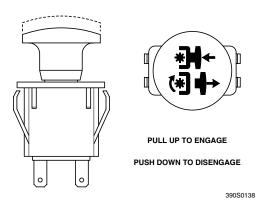
Figure 4-4. Cutter Engage Switch
