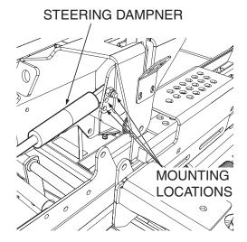
Figure 6-9. Steering Dampner Adjustment
