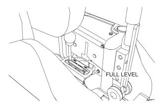
Figure 7-2. Hydraulic Oil Reservoir
