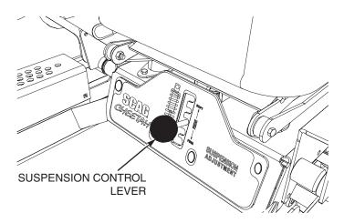
Figure 4-11. Operator Suspension Platform Adjustment
