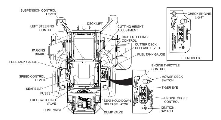
Figure 4-2. Controls and Instruments
