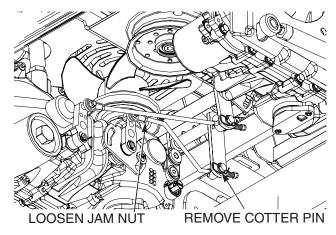
Figure 6-4. Speed Control Adjustment
