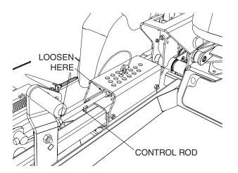
Figure 6-7. Cutter Deck Height Adjustment
