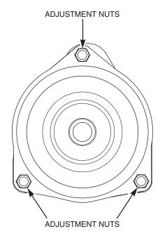
Figure 6-11. Clutch Air Gap Adjustment
