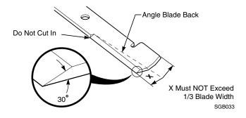
Figure 7-9. Blade Sharpening
