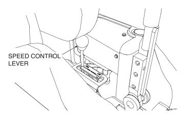
Figure 4-10. Speed Control Lever
