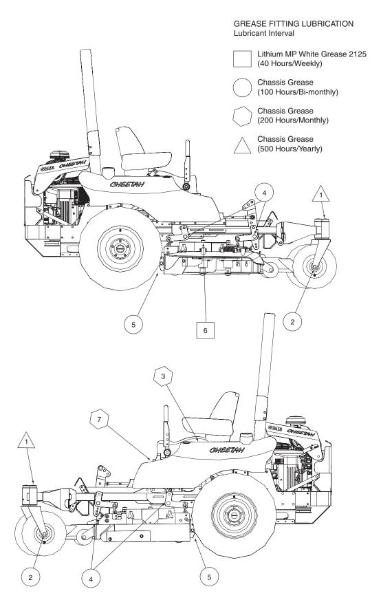
Figure 7-1. Lubrication Fitting Points
