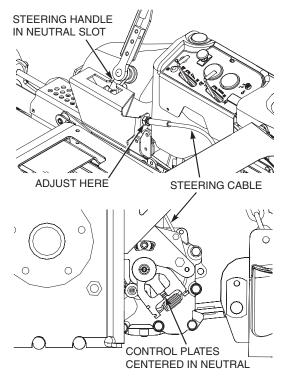
Figure 6-2. Steering Control Cable Adjustment
