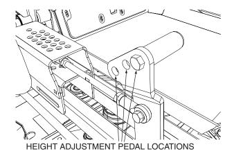
Figure 4-8. Height Adjust Pedal Locations
