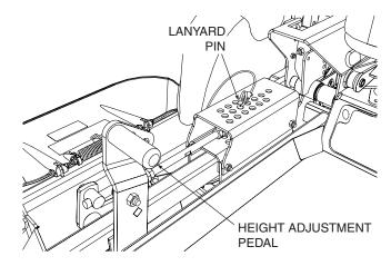
Figure 4-6. Adjusting Cutting Height
