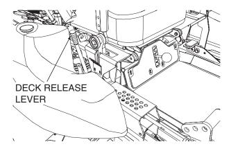
Figure 4-7. Deck Release Lever
