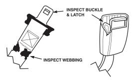
Figure 2-3. Seat Belt Inspection
