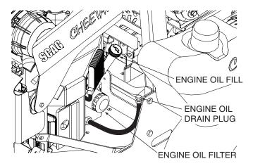
Figure 7-5. Engine Oil Fill/Dipstick, Filter and Drain Locations
