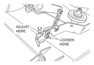
Figure 6-5. Cutter Deck Level Adjustment
