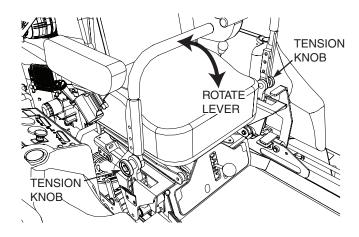
Figure 4-9. Adjusting Steering Levers
