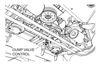
Figure 4-3. Dump Valve Control
