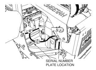
Figure 1-1. Mower Serial Number Plate Location
