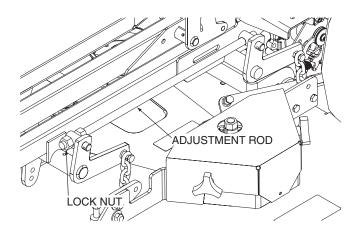
Figure 6-6. Cutter Deck Level Adjustment
