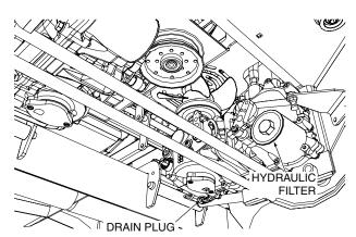
Figure 7-3. Hydraulic Oil Filter and Drain Plug
