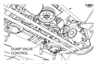
Figure 4-5. Dump Valve Control
