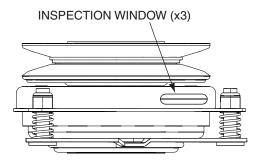
Figure 6-8. Clutch Air Gap Adjustment
