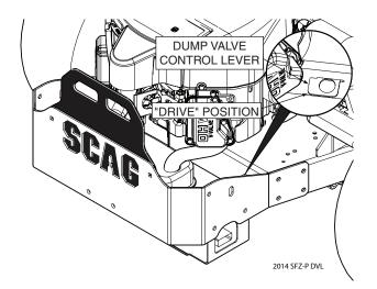
Figure 7-4. Dump Valve Control Lever
