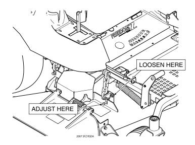
Figure 6-6. Cutter Deck Pitch Adjustment
