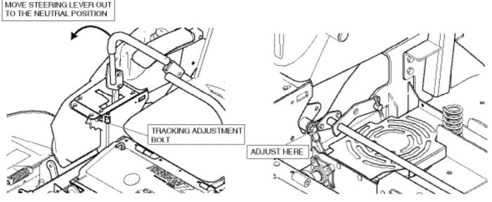
Figure 6-3. Steering Control Rod Adjustment
