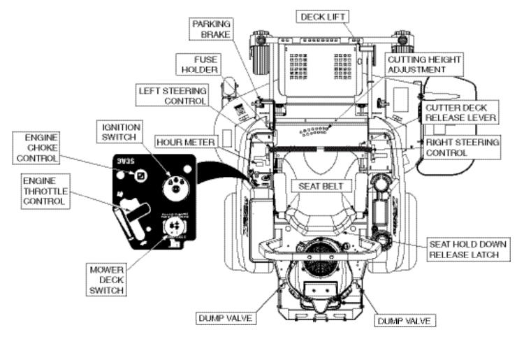
Figure 4-1. Controls and Instruments
