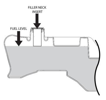
Figure 7-6. C.A.R.B. / EPA Phase 3 Fuel Level
