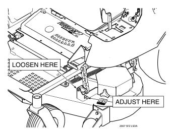
Figure 6-5. Cutter Deck Pitch Adjustment
