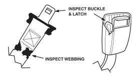
Figure 2-1. Seat Belt Inspection
