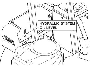
Figure 7-1. Hydraulic System Oil Level
