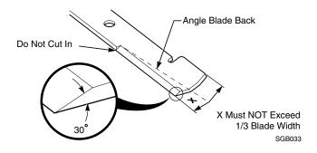
Figure 7-8. Blade Sharpening
