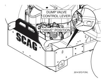
Figure 4-2. Dump Valve Control
