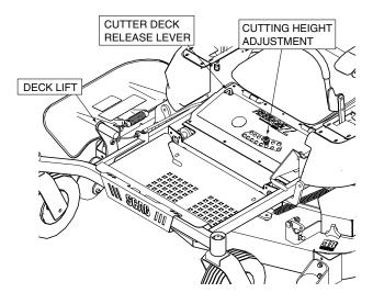
Figure 4-4. Adjusting Cutting Height
