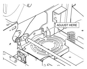
Figure 6-2. Brake Rod Adjustment
