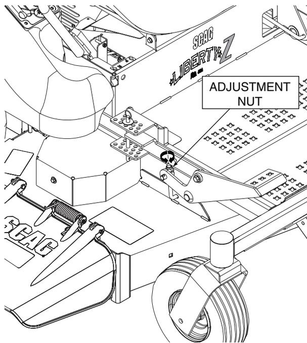
**Figure 6-6. Cutter Deck Pitch Adjustment**
