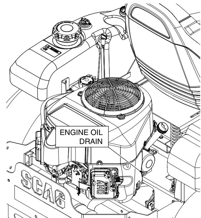
Figure 7-5. Oil Fill / Dipstick, Oil Filter, Oil Drain
