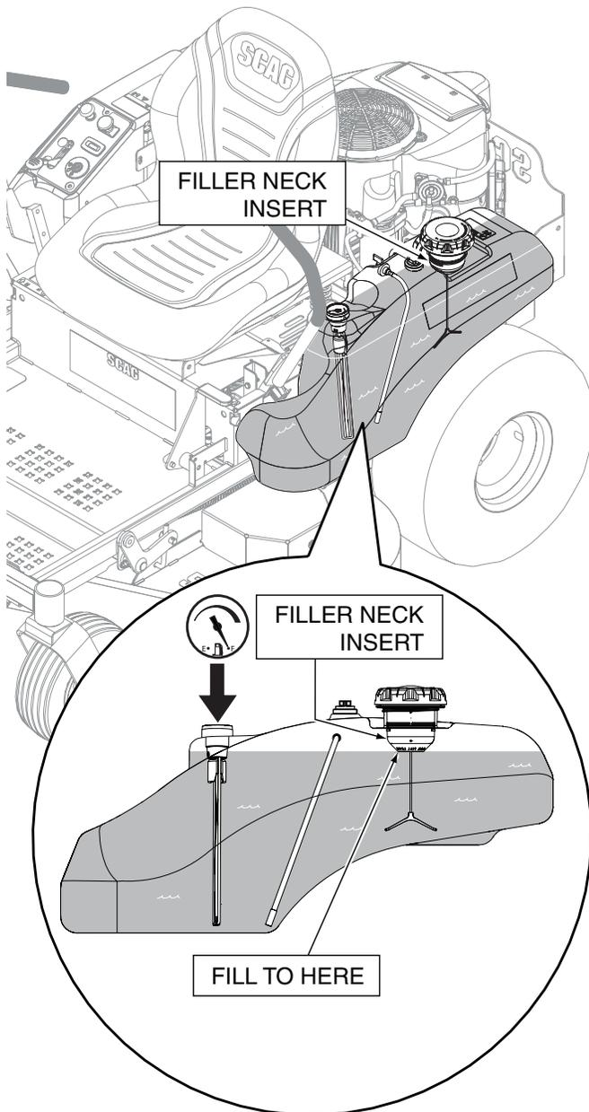
**Figure 7-6. Fuel Tank Fill Level**
