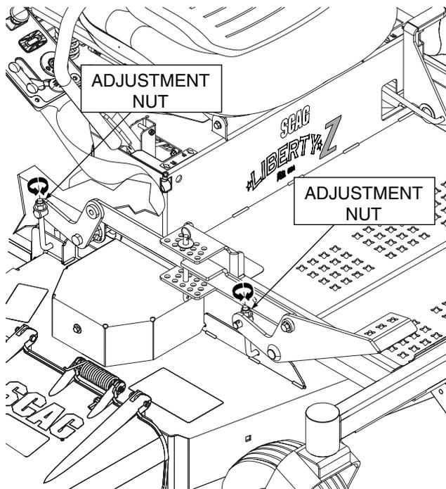
**Figure 6-8. Cutter Deck Height Adjustment - Right Side**
