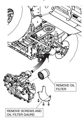
Figure 7-1. Hydraulic Oil Filter and Drain Plug
