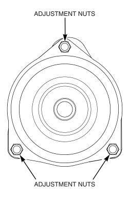
Figure 6-10. Clutch Air Gap Adjustment
