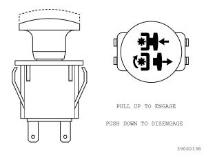
Figure 4-3. Cutter Engage Switch
