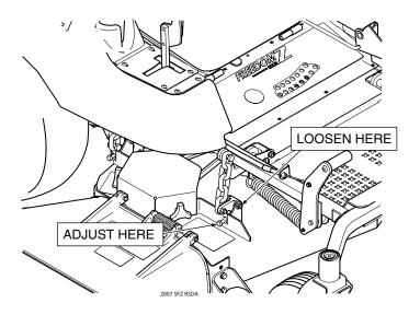
Figure 6-6. Cutter Deck Pitch Adjustment
