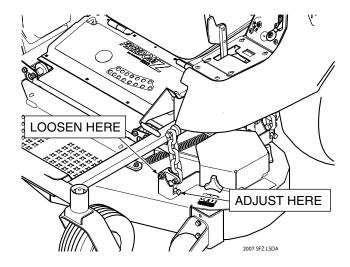
Figure 6-5. Cutter Deck Pitch Adjustment
