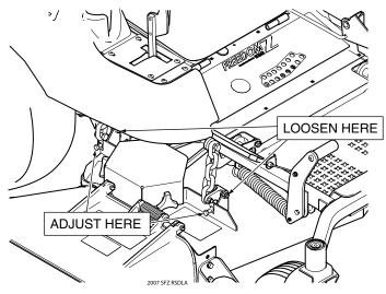
Figure 6-7. Cutter Deck Height Adjustment
