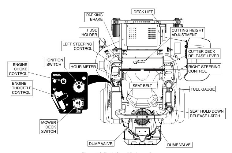
Figure 4-1. Controls and Instruments
