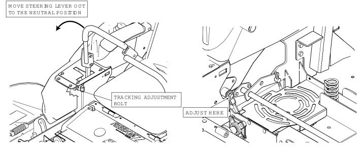
Figure 6-3. Steering Control Rod Adjustment
