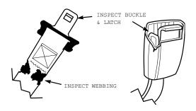
Figure 2-2. Seat Belt Inspection
