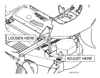
Figure 6-4. Cutter Deck Level Adjustment
