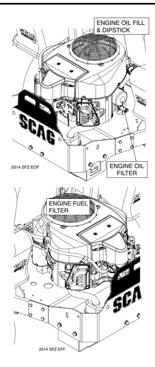
Figure 7-5. Oil Fill / Dipstick, Oil Filter, Fuel Filter
