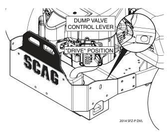
Figure 4-2. Dump Valve Control
