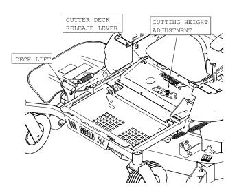
Figure 4-4. Adjusting Cutting Height
