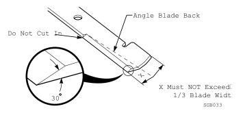
Figure 7-8. Blade Sharpening
