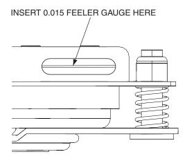
Figure 6-9. Clutch Air Gap Adjustment
