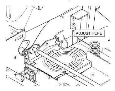
Figure 6-2. Brake Rod Adjustment
