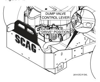
Figure 7-4. Dump Valve Control Lever
