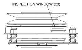
Figure 6-8. Clutch Air Gap Adjustment
