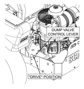
Figure 4-4. Dump Valve Control
