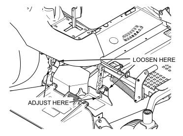
Figure 6-7. Cutter Deck Height Adjustment
