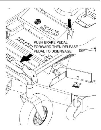
Figure 4-3. Releasing the Parking Brake
