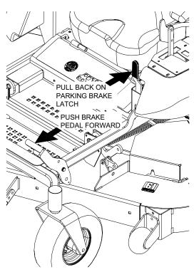
Figure 4-2. Engaging the Parking Brake
