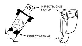
Figure 2-4. Seat Belt Inspection
