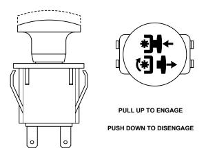
Figure 4-5. Cutter Engage Switch
