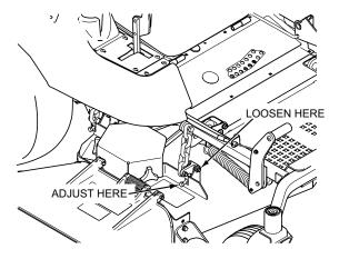
Figure 6-6. Cutter Deck Pitch Adjustment
