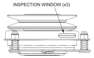
Figure 6-8. Clutch Air Gap Adjustment
