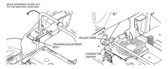
Figure 6-3. Steering Control Rod Adjustment
