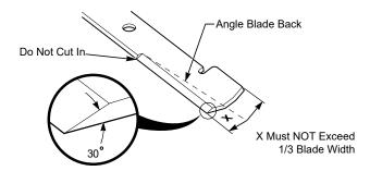
Figure 7-9. Blade Sharpening
