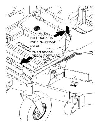
Figure 6-1. Brake Adjustment
