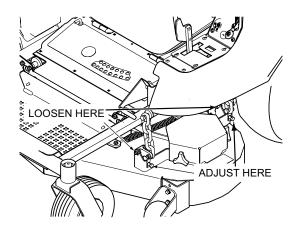
Figure 6-4. Cutter Deck Level Adjustment
