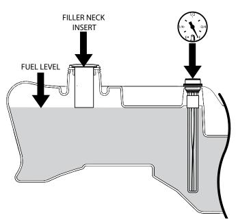
Figure 7-7. C.A.R.B. / EPA Phase 3 Fuel Level
