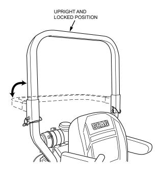
Figure 2-2. Foldable Roll-Over Protection Structure
