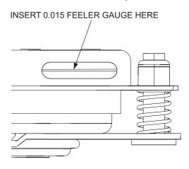
Figure 6-9. Clutch Air Gap Adjustment
