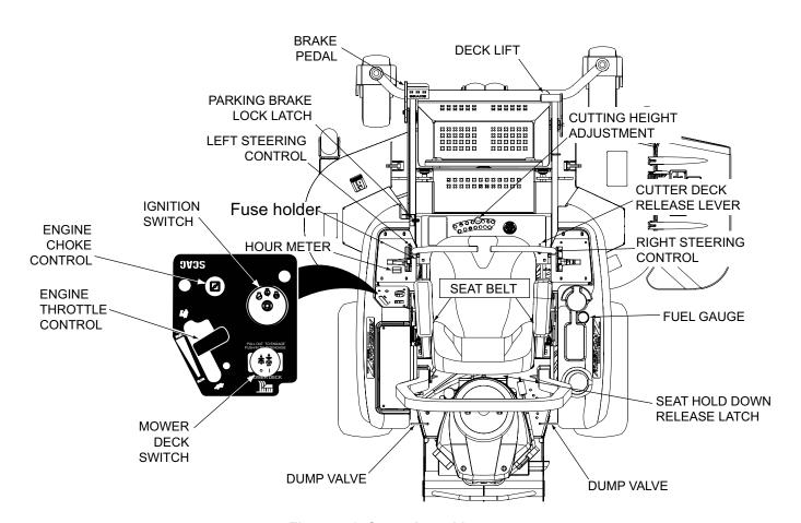
Figure 4-1. Controls and Instruments
