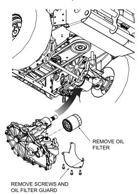
Figure 7-2. Hydraulic Oil Filter and Drain Plug
