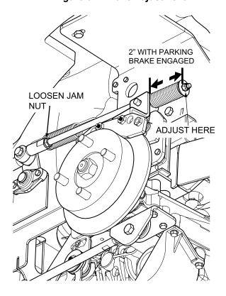
Figure 6-2. Brake Rod Adjustment
