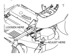
Figure 6-5. Cutter Deck Pitch Adjustment
