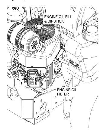
Figure 7-6. Oil Fill / Dipstick, Oil Filter
