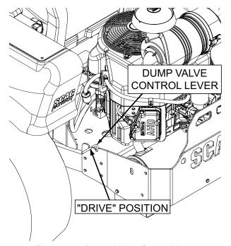
Figure 7-5. Dump Valve Control Lever
