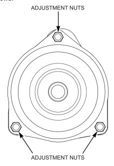
Figure 6-10. Clutch Air Gap Adjustment
