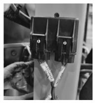
Figure 6-7. Engine Fuses
