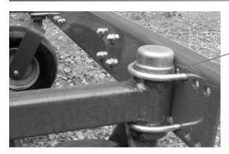
Attach Mounting Bar to front of mower/rider by laying bar against front caster arms and slipping one U-bolt around top and bottom of each of the two front caster arm bosses and through corresponding holes in bar. Be sure bar is centered.
