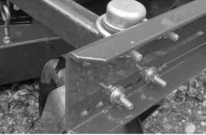
Secure each U-bolt to bar with one 3/8" flat washer, lock washer and nut on each of the eight threaded ends. Tighten all hardware securely.
